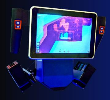
Capture and document evidence with precision using LABview, an autonomous camera and video system for examination of body fluids, hair, fibers, GSR, and fingerprints.
